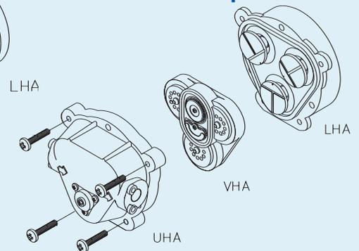
**UHA:** Upper Housing Assembly • **VHA:** Valve Housing Assembly • **LHA:** Lower Housing Assembly
