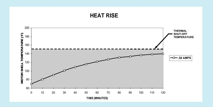
All of the pump models in the Performance Data and Heat Rise charts are in the shaded area, meaning they are capable of sustaining continual running, at any of the above listed pressures, without shutting down to allow the motor to cool. To conserve wearing parts, however, the pump should only operate as needed.
