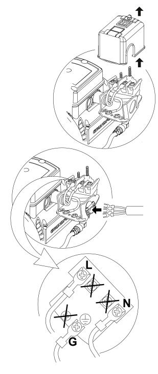
Fig. Connecting a power cable
