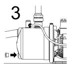
Fig. Draining the JP PS pump
