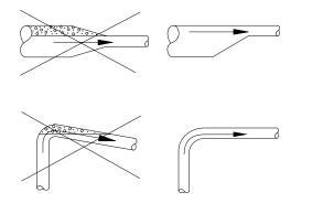
Fig. Recommended pipe installation to avoid friction and air pockets
