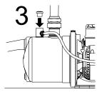
Fig. Priming the JP PS pump
