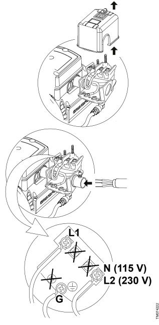
Fig. Connecting to residential hard wiring, 115 or 230 V
