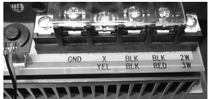
1Ø - 2W/3W Wires to Motor
